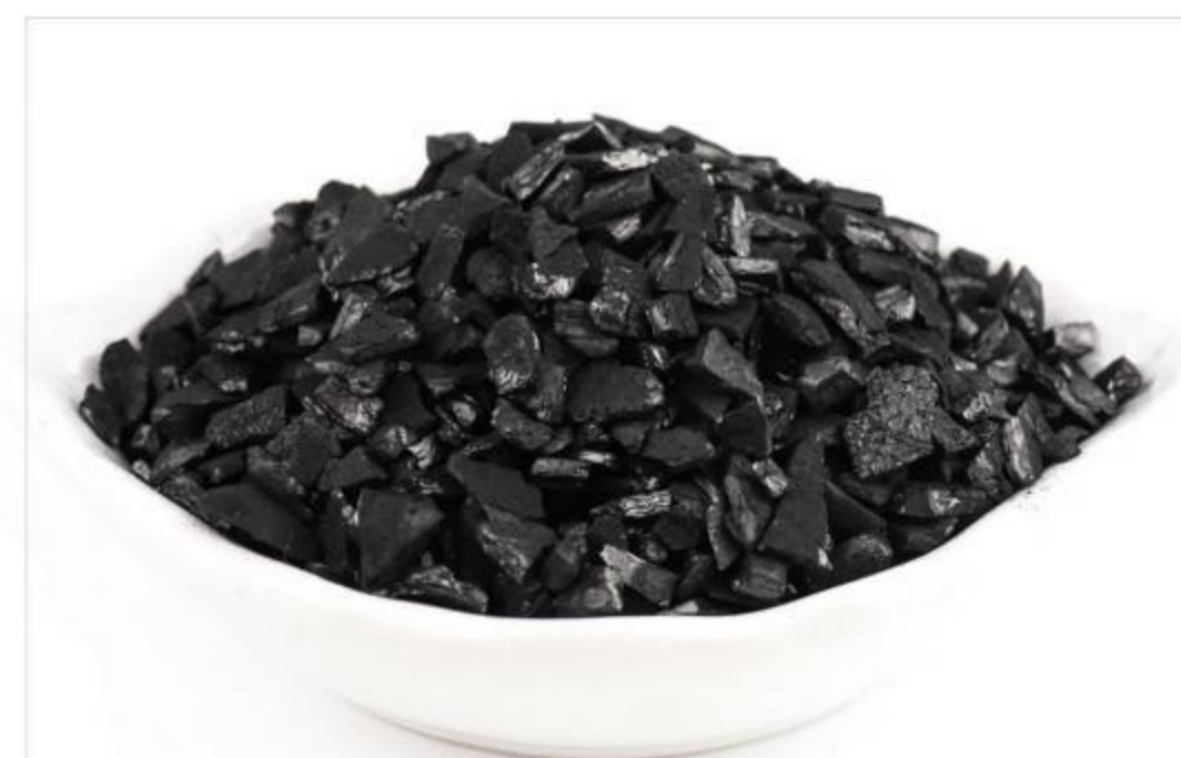
① granular activated carbon
